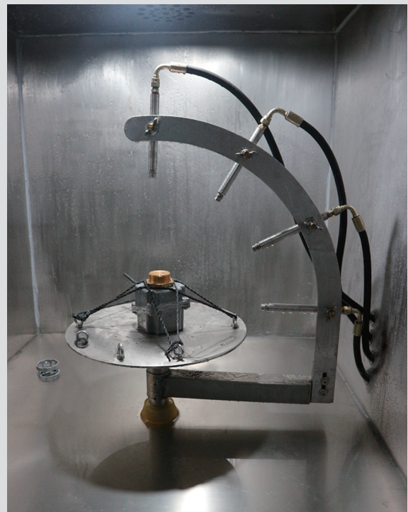
Enclosure during IPx9k test
